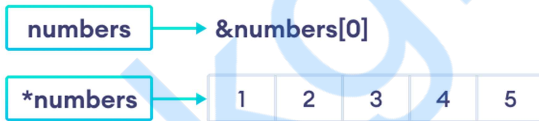
Figure: Array and Pointer
